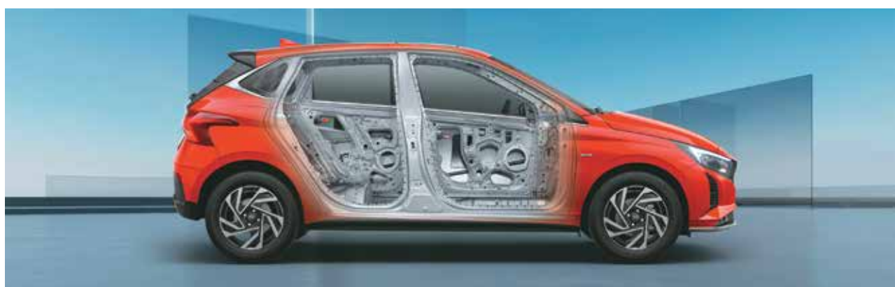
Strong body structure (with AHSS and HSS)
